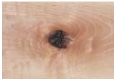
UNSOUND KNOT: A circular area that once formed the base of a branch or twig and has a pith centre. (In some cases the wood may be missing).
