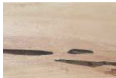
GRUB HOLES: Holes larger than \frac{1}{4} "
